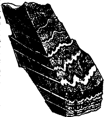
Sketch (by Du Noyer) of a block of variegated slate from Devil's Glen, Co. Wicklow. The crumpled bands mark the bedding, and the fine perpendicular striae in front are the cleavage planes; the fine lines on the darkened side merely represent shadows, and must not be taken for planes of division in the rock. It will be observed that the cleavage planes do not pass through the white bands.
