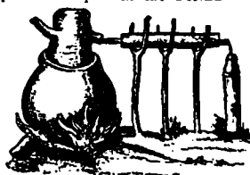
FIG. 4.—Ancient form of Still, used in Tahiti.
