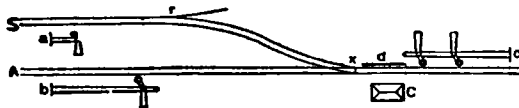
FIG. 5.—Interlocked signals (American practice, signals at right track, and arms at right of post).
